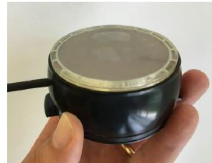
Coupling pad attached to transducer
