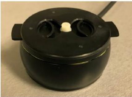
Transducer showing clip mechanism
